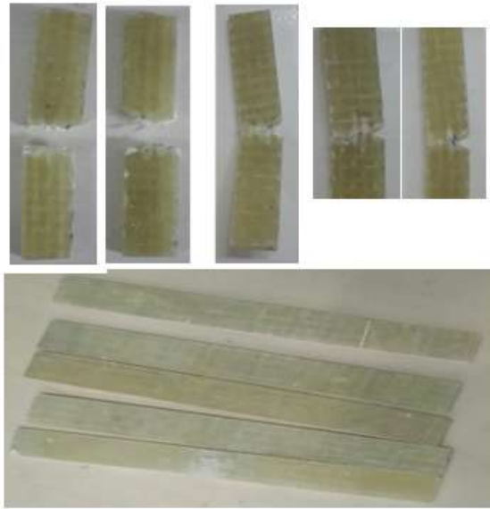
Fig. 2 Three-point bending test specimens
